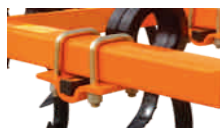
U clamp for attachment & adjustment of tyne
